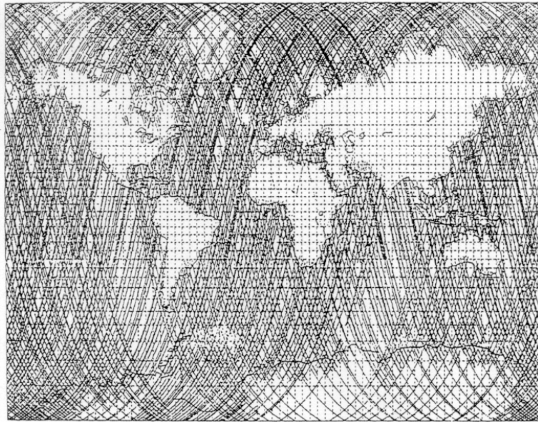
Figure 5 - spatial coverage of ERS 1&2: ground track during its 35-day cycle
