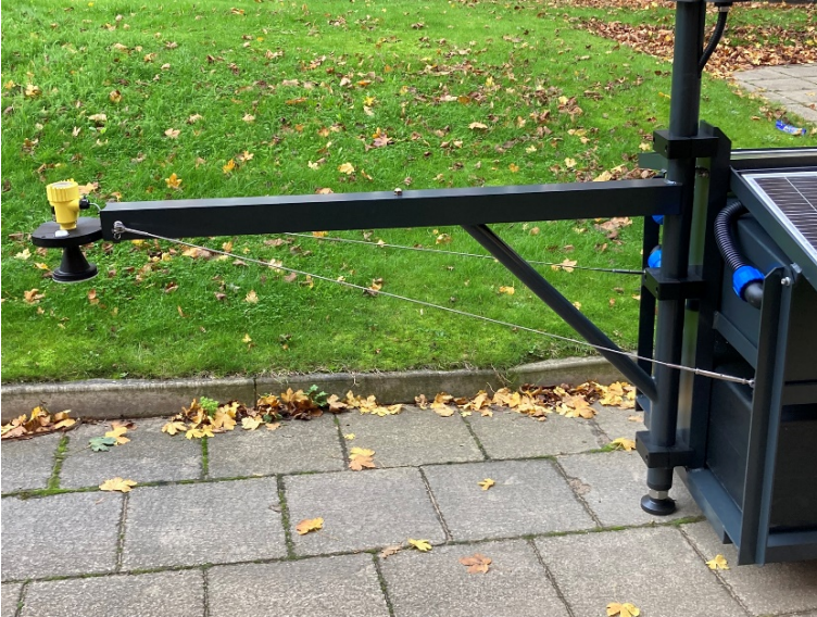
Figure 10. Radar arm tensioning (guy) wires.
