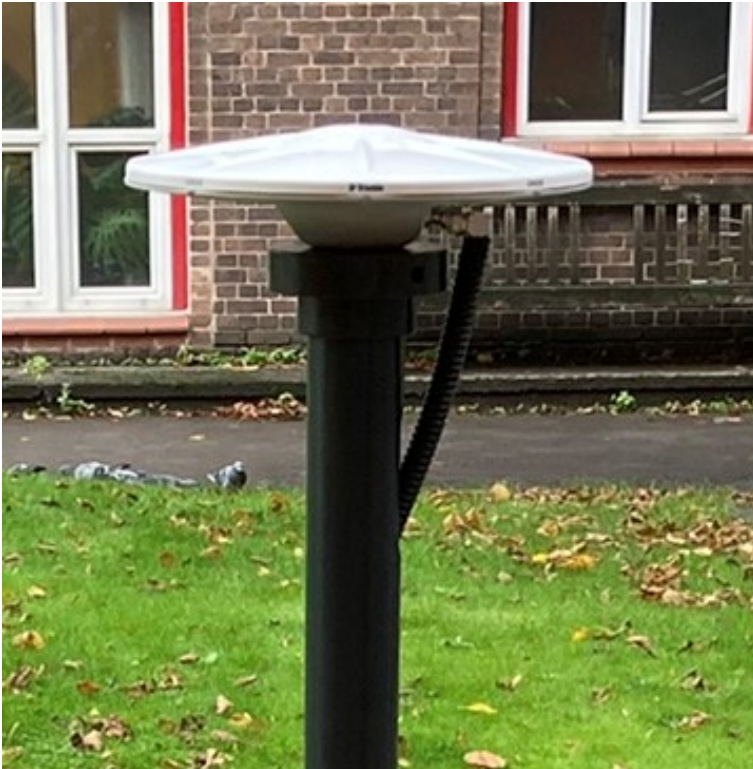
Figure 6. GNSS antenna and cable fitted onto the mast.
