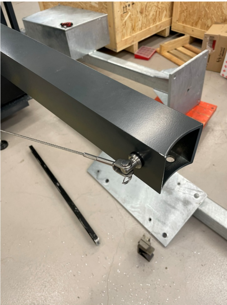
Figure 11. Guy wires attached to radar arm.
