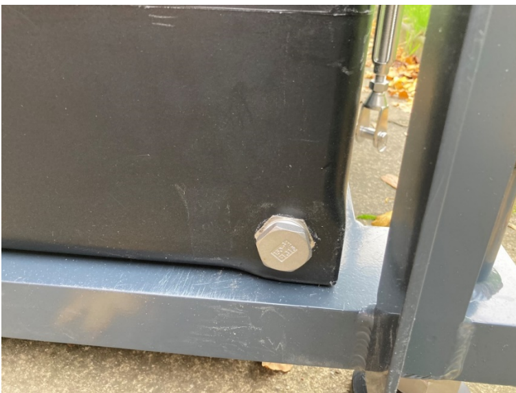
Figure 50. Ballast tank drain plug.
