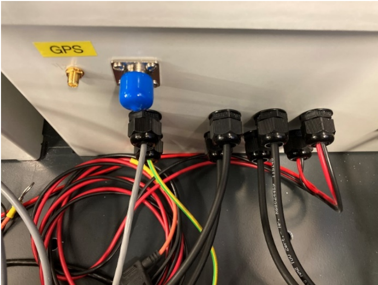
Figure 23. Logger enclosure connectors. N type connector (blue) is not used.
