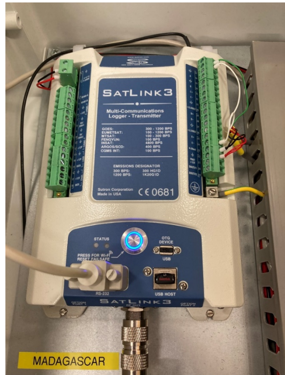
Figure 33. Connect the serial data lead to the Satlink3 logger if a mobile data connection is available.
