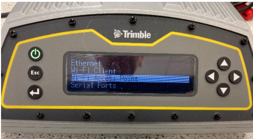
Figure 48. Wi-Fi Access Point.
