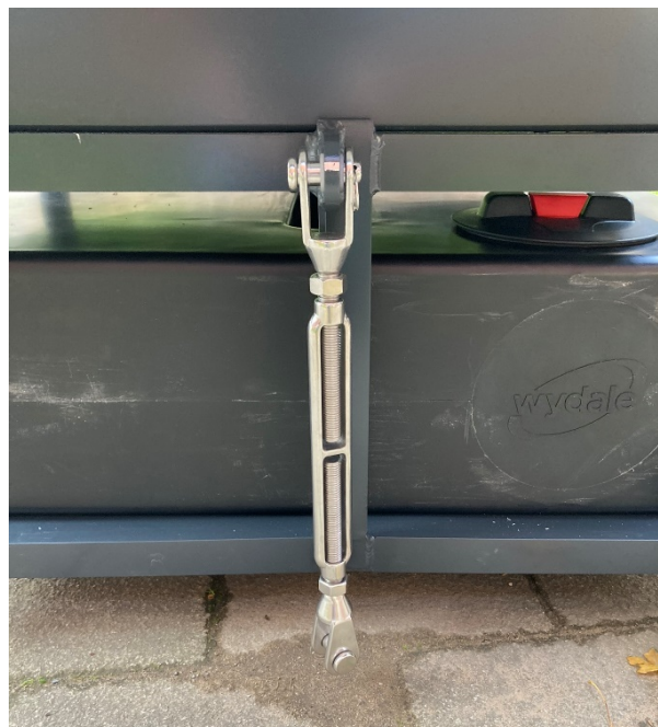
Figure 42. Water tank filling point and turnbuckle anchoring point.
