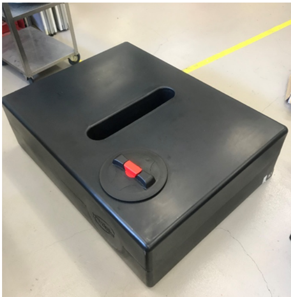
Figure 41. Plastic water ballast tank.
