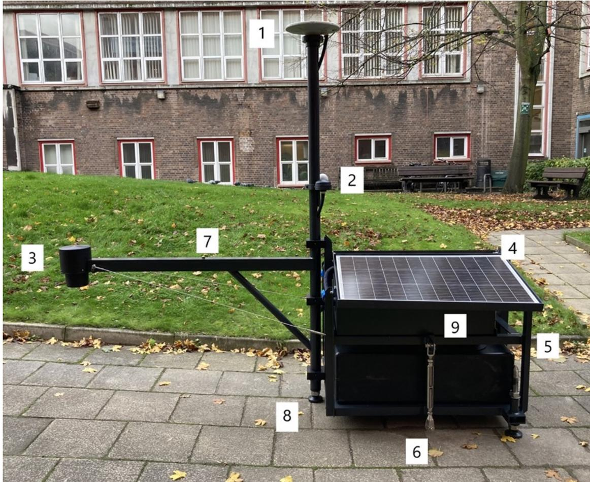
In addition to the radar gauge [3] the portagauge also has a geodetic quality GNSS unit [Trimble Alloy] and GNSS Antenna [1].
