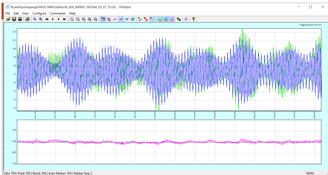
Figure 6. Portagaugue Sea Level Data on TASK application (June to September 2023). In the top panel the green line gives the recorded sea level, and the blue line the tidal prediction. The magenta line in the bottom panel gives residual sea level (recorded minus tidal prediction).
