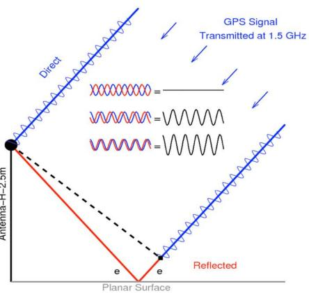
GNSS signals suffer from reflections from surfaces near to the antenna. This is called multipath and interference occurs between the direct and reflected signal If we understand the interference effects on the signal for instance when the reflection is off a flat surface such as a body of water then we can use this to extract information about these surfaces.
