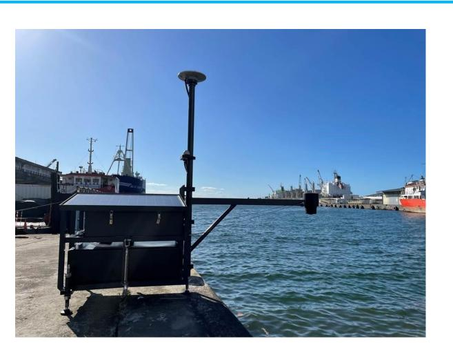
In addition to the radar gauge the portagauge also has a geodetic quality GNSS unit [Trimble Alloy] and GNSS Antenna.
