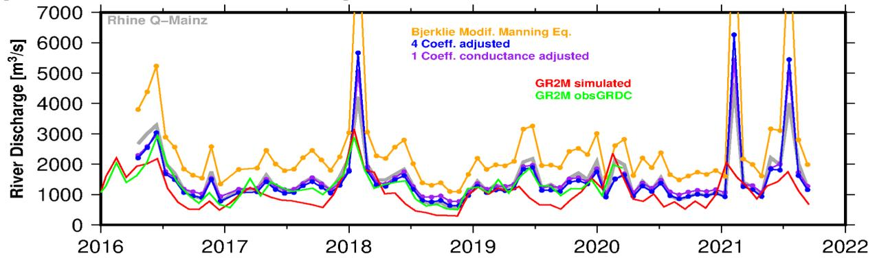
Figure 2.5 River discharge derived in Mainz from the three approaches and from the GR2M model
