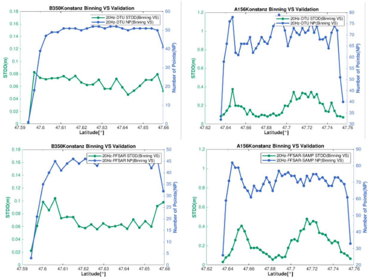
Figure 2.4 Lake of Constance. Accuracy as STDD of altimetric and gauge water height (green) and number of points per bin (blue) from the DTU products (top) and from in-house FF-SAR (bottom). Ground tracks SA156 and SB350 in Fig. 2.1.
