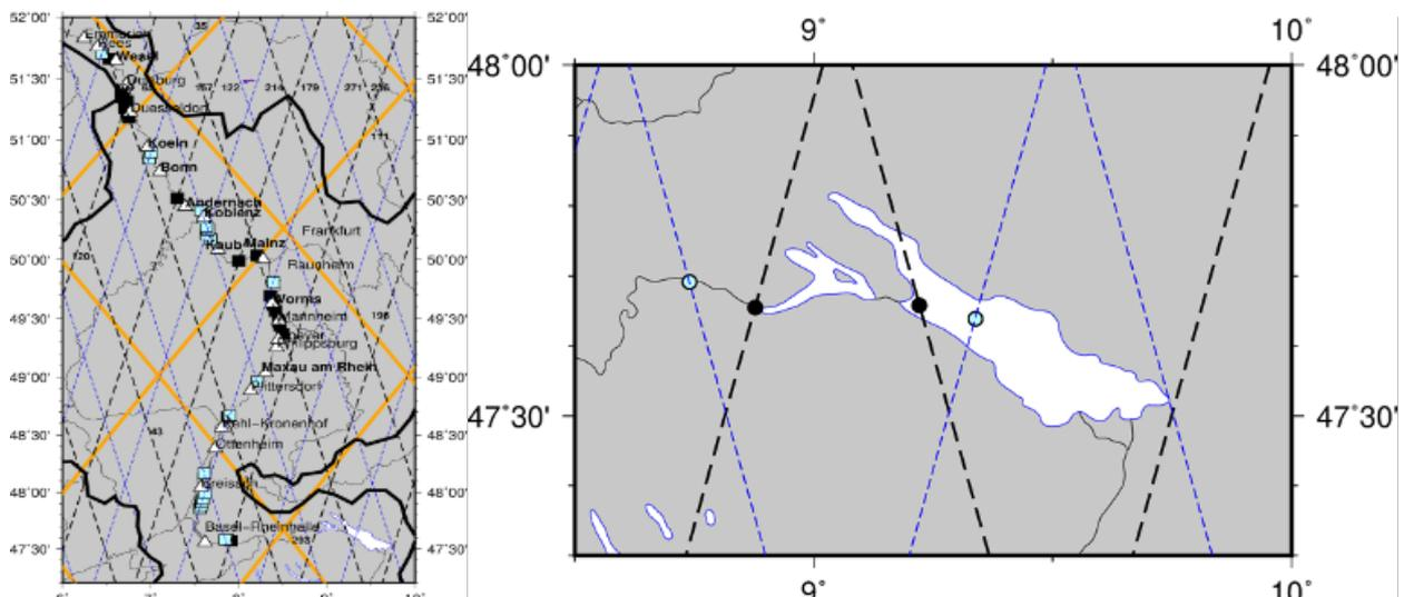
Figure 2.1. Inland Water case study on the River Rhine with Sentinel-3A/3B/6A ground tracks (black, blue, orange) and locations of fiducial reference data from operational tide gauges of the BfG network (left). Lake of Constance (right).
