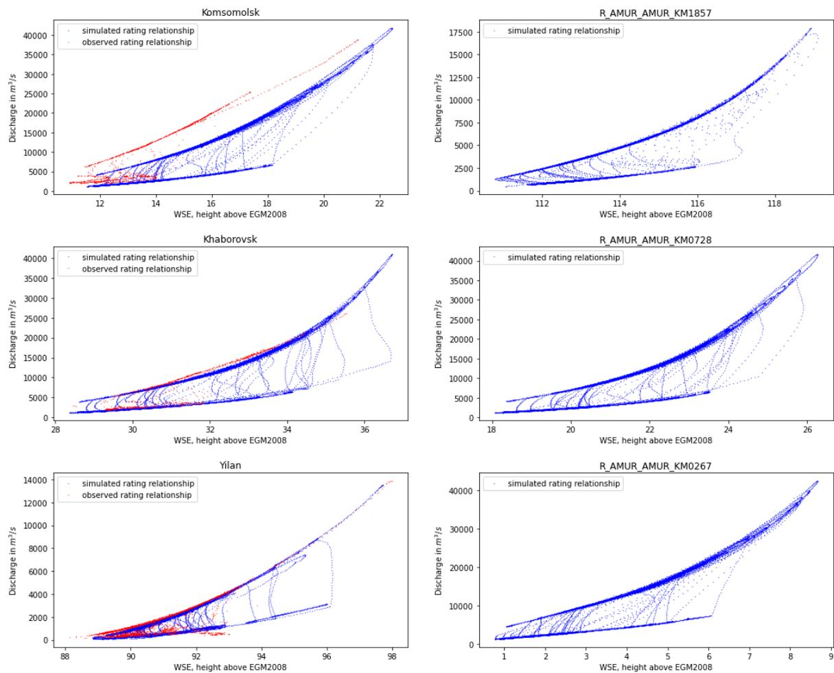
Figure 5.2: Simulated and observed rating relationships at selected in-situ stations (left) and virtual stations (right) on the Amur River
