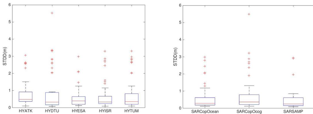
Figure 2.2 Boxplot of STDD at the 42 VGs for unfocused SAR Hydrocoastal (left) and for standard and dedicated products (right). The best accuracy is from SARvatore SAMP
