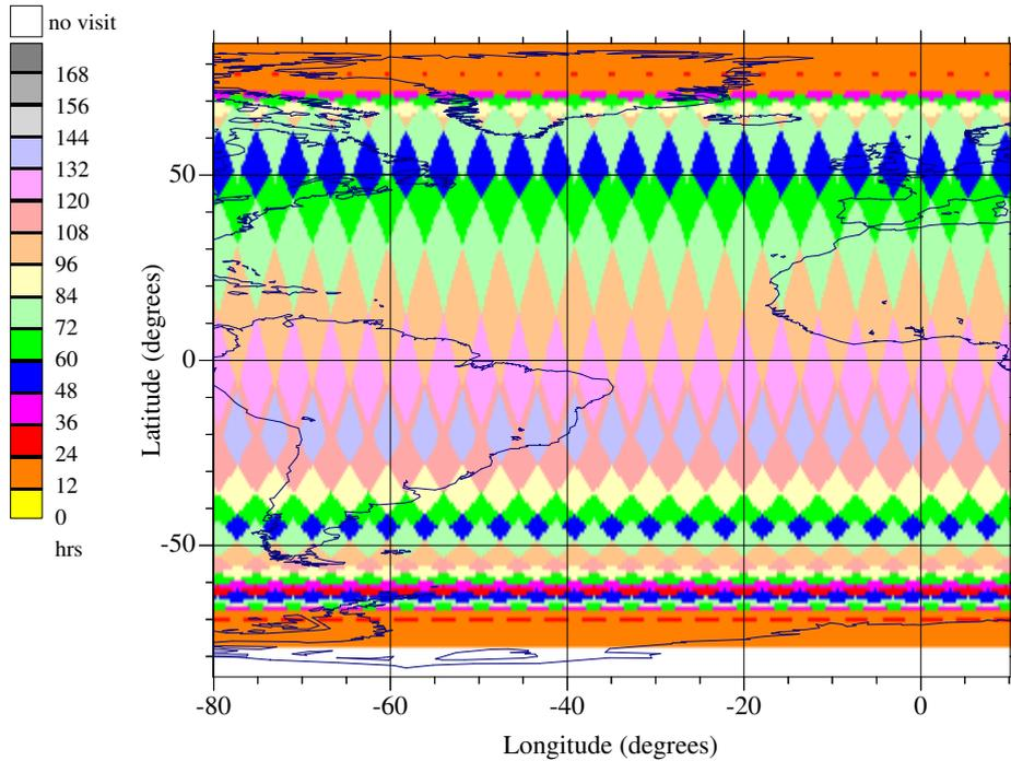
Figure B-11. Maximum Revisit Interval (803 km 80° orbit, 20–50° incidence swath)
