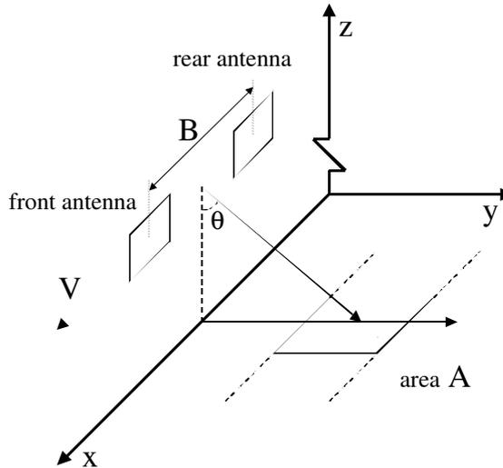
Figure 3-1. Schematic of ATI operation.
