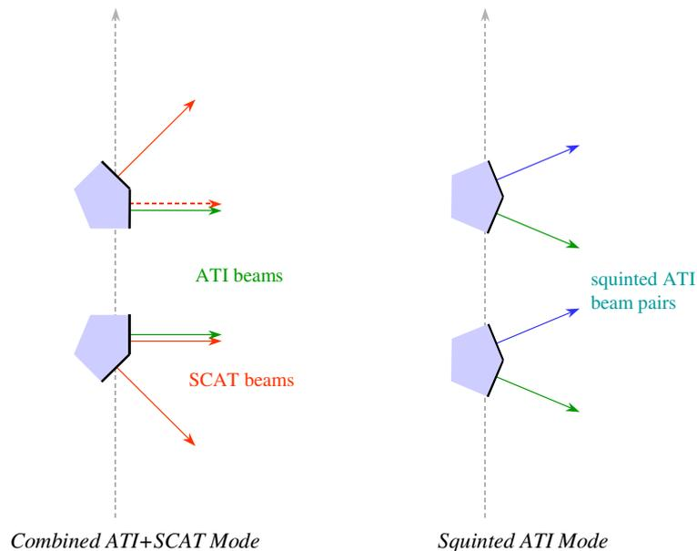
Figure 3-7. Formation with Two Beams per Satellite
