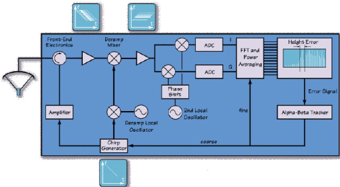
Figure 2-1. Block Diagram of RA-2 (single channel only shown)
