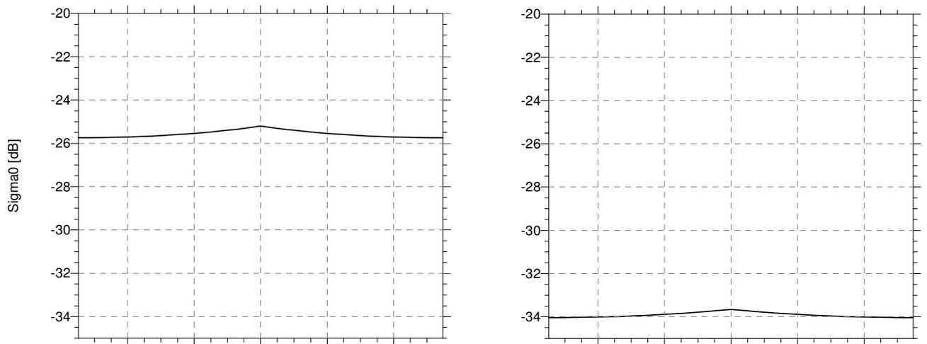
Figure B-8. Along-Track Variation of NESZ for Subswaths 1 (left) and 7 (right)
