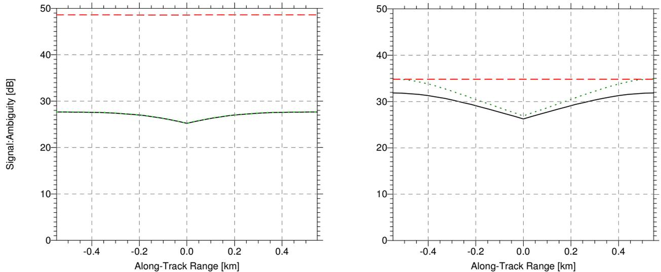
Figure B-9. Along-Track Variation of Ambiguities for Subswaths 1 (left) and 7 (right)
