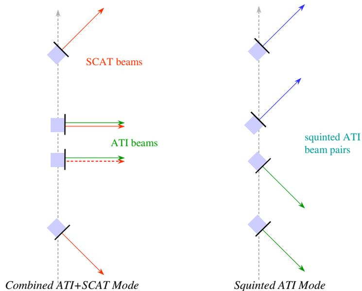
Figure 3-6. Formation Combining ATI and Scatterometer Modes
