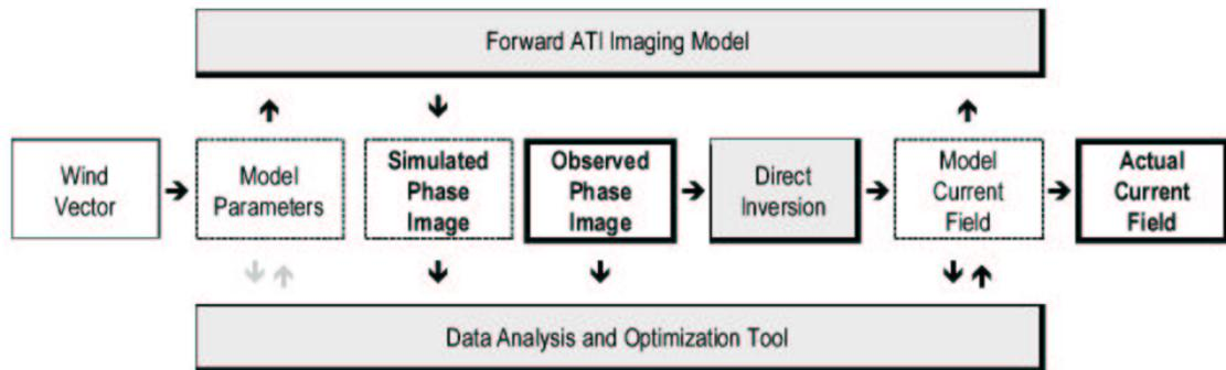
Figure 3-2. Schematic for the retrieval of surface currents by along-track interferometry (from Romeiser et al. [15]).
