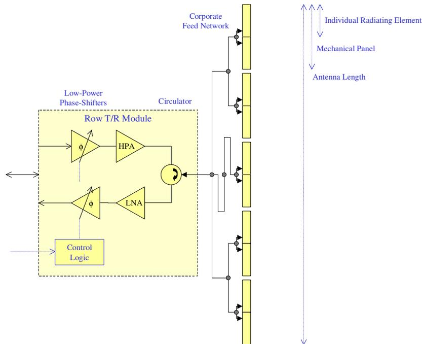
Figure B-13. Row-Based Architecture – Distribution within each Row
