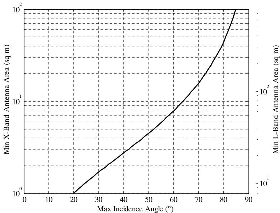
Figure B-3. Minimum Antenna Area versus Operating Incidence, 800 km Altitude
