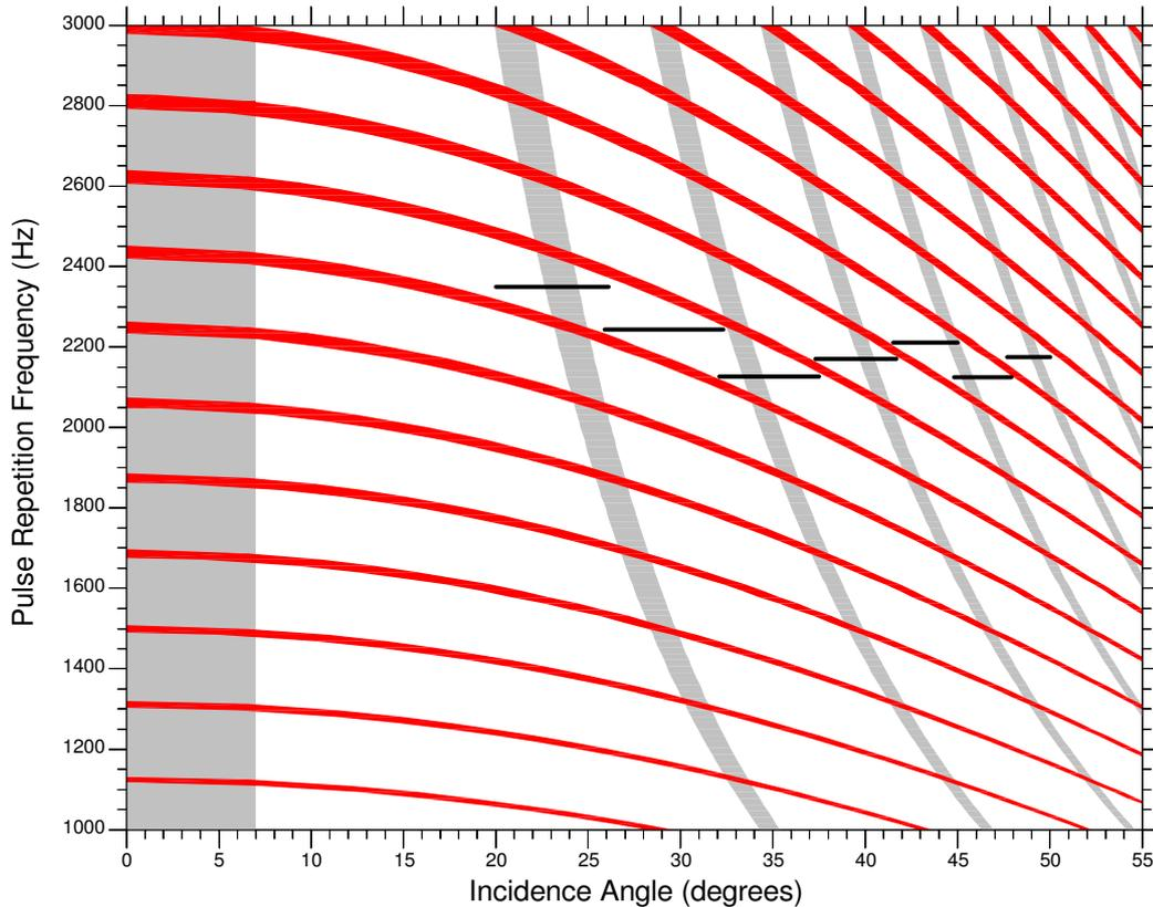
Figure B-5. Pulse Timing Diagram showing all Seven Subswaths
