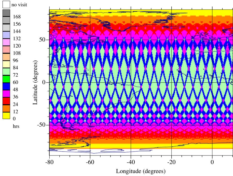
Figure B-10. Mean Revisit Interval (803 km 80° orbit, 20–50° incidence swath)
