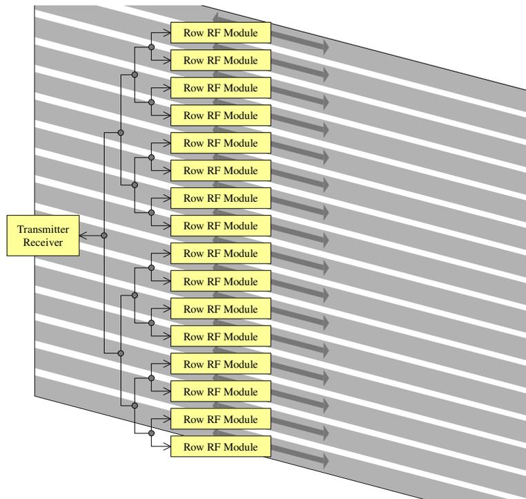
Figure B-12. Row-Based Architecture – Feeds to the Antenna Rows
