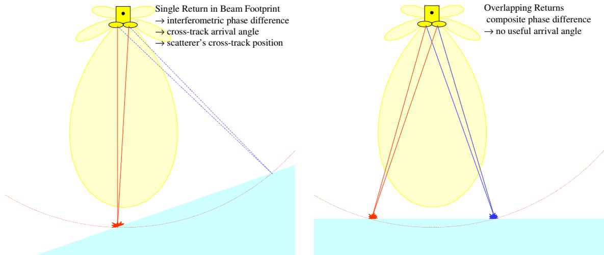
Figure 2-2. Interferometric Returns over Tilted and Horizontal Surfaces
