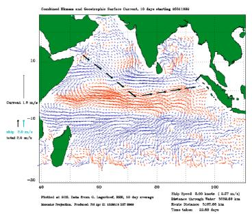
Figure 5. Ship routing trial for 05/11/98 (NE Monsoon). The ship (green) and combined ship and current vectors (black) are indicated by the heavy arrows. The underlying current fields are indicated by the red (east flowing) and blue (west flowing) arrows.
