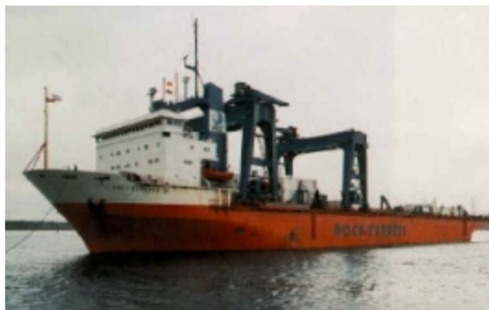
**Figure 2.19 The Dockwise Cable Laying Vessel, Dock Express 20.**
