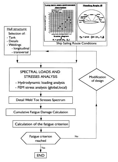
Figure 2.2 Direct Calculation Fatigue Analysis Procedure Flow Chart.
