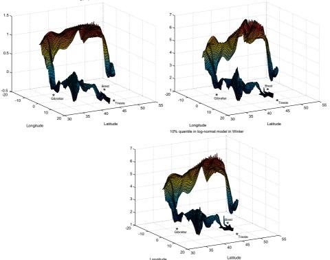
Figure 2.6 Analysis of satellite altimeter significant wave height data along the Rotterdam — Trieste route. Top left — Mean of log(Hs)for winter, Top Right- Estimated 10% Hs quantile for winter, Bottom -10% Hs quantile from a log-normal model generated from reconstructed data.
