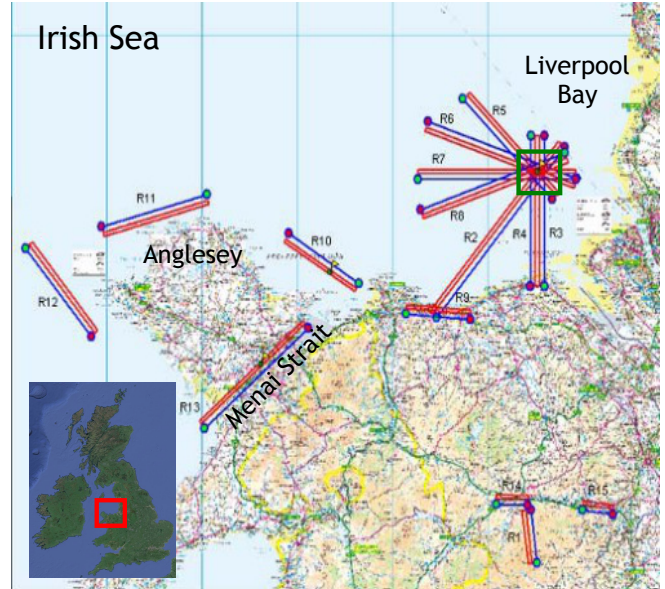
Fig. 1. Location of Wavemill airborne proof-of-concept flights over the Irish Sea/Liverpool Bay/Anglesey area off the west coast of the UK. The various Wavemill runs are denoted as R2, R3, .... The dark green square indicates the data in the star pattern centred over the Mersey Bar Light which are considered in this paper.
